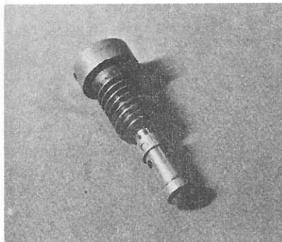
5.11c Idle jet size location (DFAV type)
