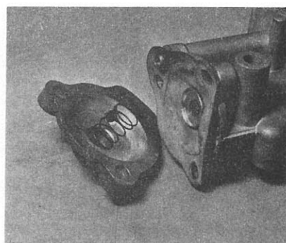
5.35 Removing the diaphragm cover (DFAV type)
