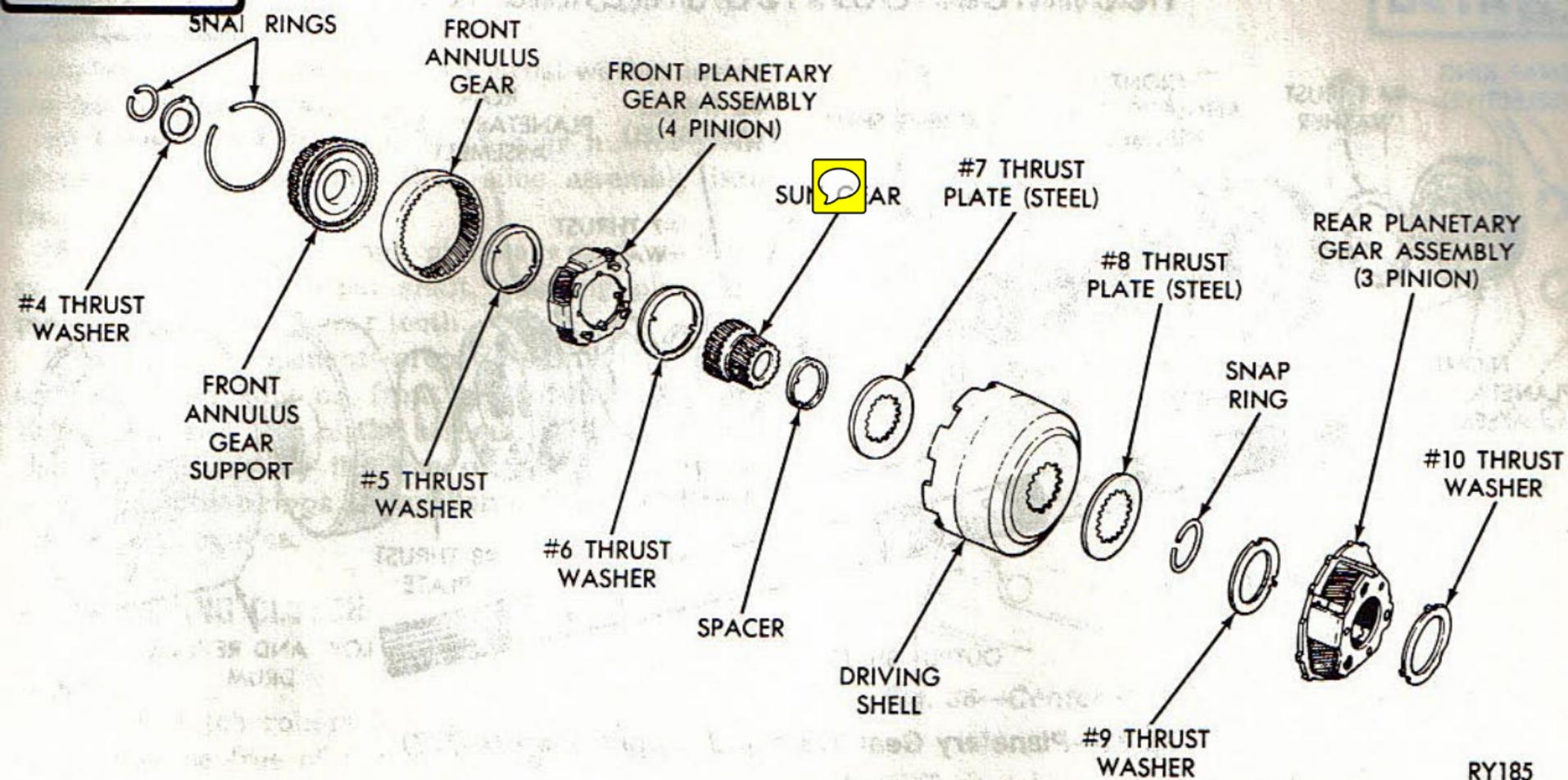
Fig. 33—Wide-Ratio Planetary Gear Train
