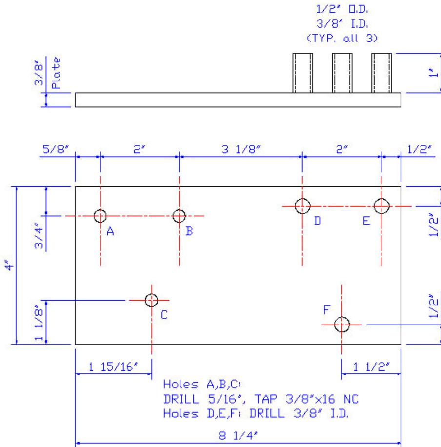
The above template will provide you with the adapter needed to pull this off. Below are a few pics of the adapter.
