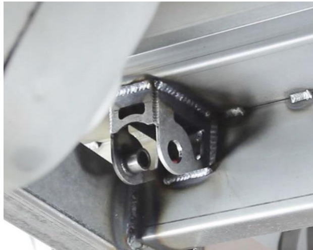
Figure 6 – Weld Upper Shock Mounts
