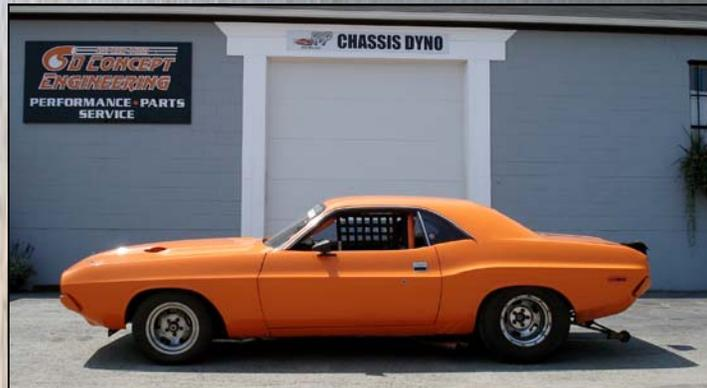
Our Challenger has been our prototype vehicle for all of our supercharger systems. Back in 1995, it originally started as a small block 360cid with a P600B blower. It has since morphed into a big block car running 8.50's at 158 mph using one of our custom big block blower kits.
