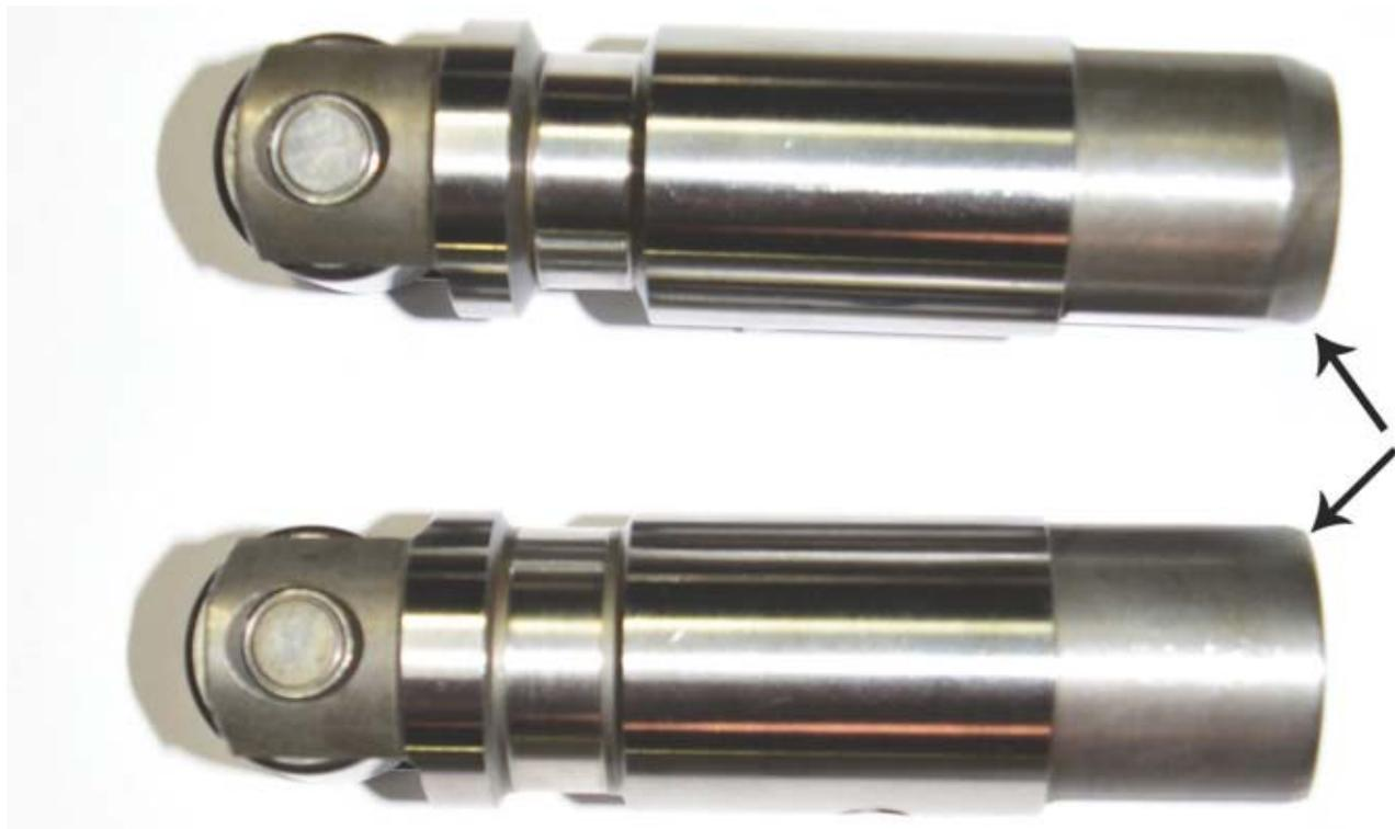
The VVT lifters are chamfered on top for easier installation in the yoke, so they're easy to identify. They were modified internally to accommodate the high lift cams used in these engines, too.
