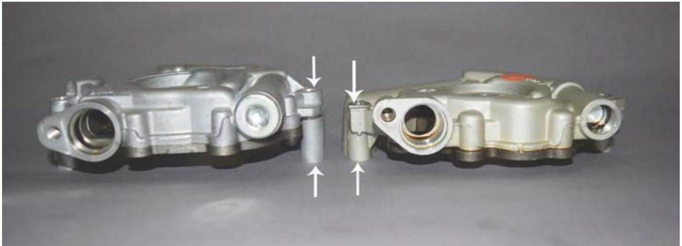
The new oil pump housing is thicker and it has a bigger pickup tube because the output was increased by 22% in order to supply enough oil for VVT. It sits up higher than the old one, too, because the crank gear was moved out further on the snout.
