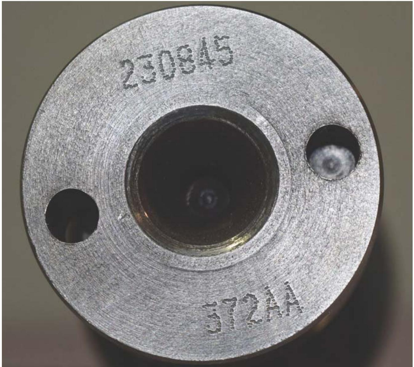
The last three digits of the part number and suffix are stamped in the back of the rear cam journal.
