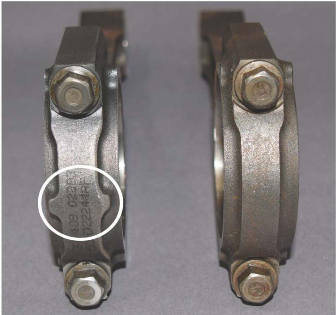
The new rods were redesigned stronger because the VVT motors make more horsepower. Look for the tabs that stick out on both sides of the balance weight.
