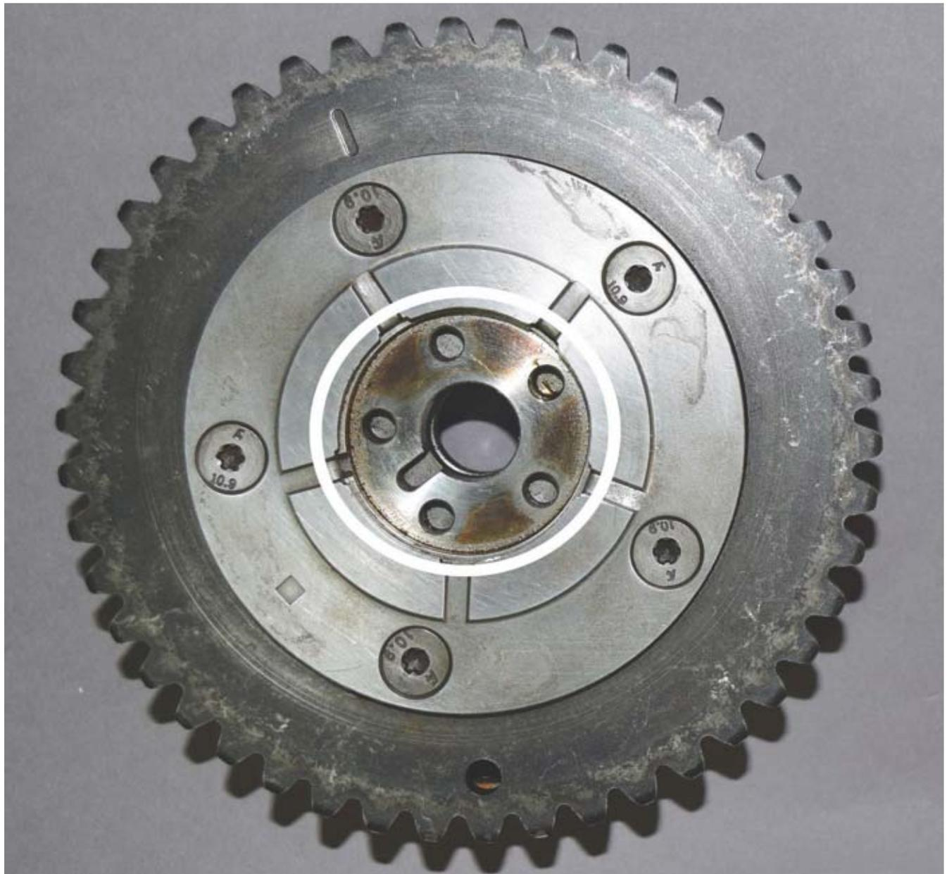
The oil control valve provides pressurized oil to the phaser thru these five passages that are aligned with the corresponding holes in the cam.
