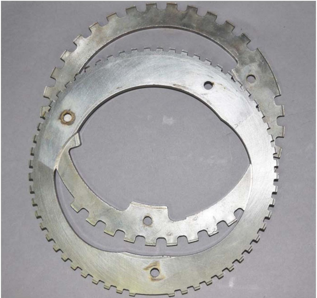
The crank sensor for the VVT motor has 58 notches instead of the 32 notches that were used on the original engine that had NGC.
