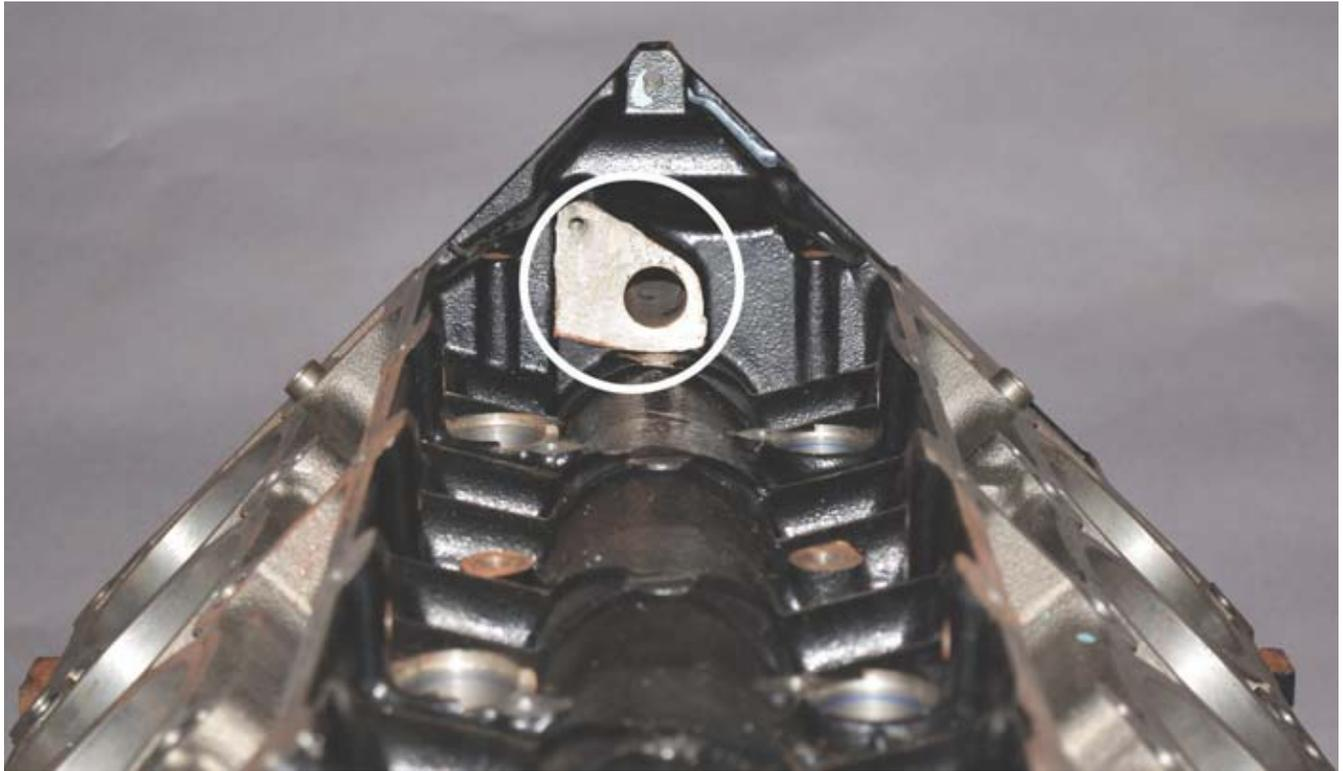
The oil control valve that directs the oil to the phaser through the front cam journal is bolted to a machined pad on the back of the timing cover.
