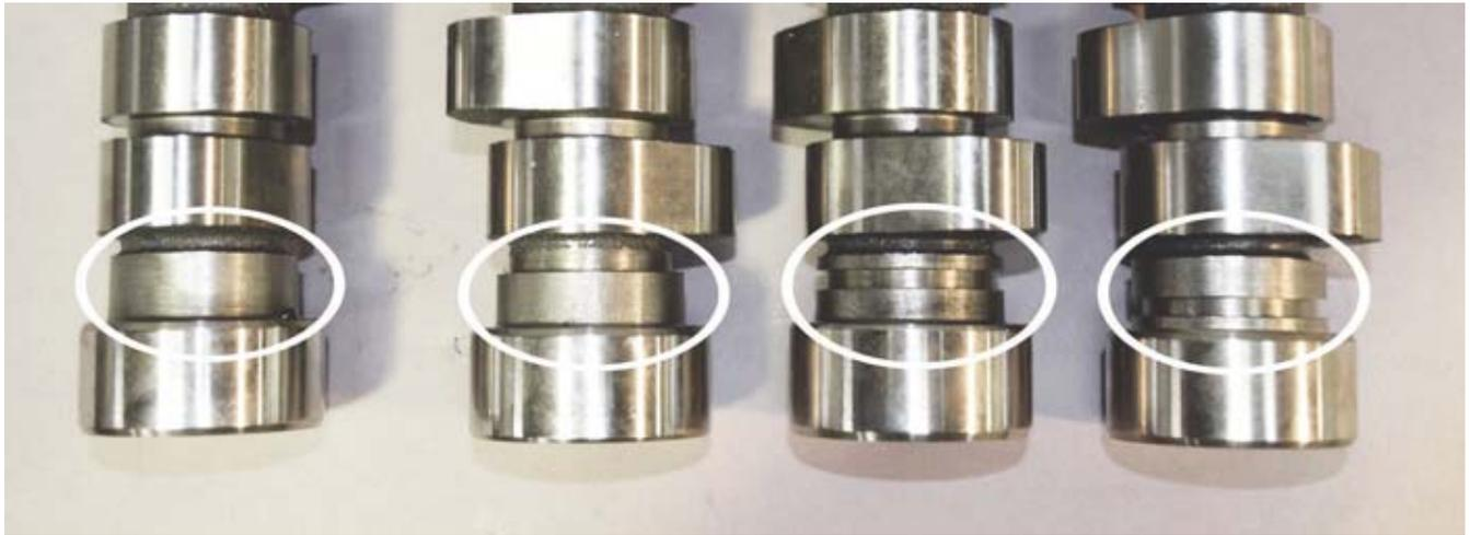
You can identify the cams by the location of the grooves machined in the barrel in front of the back journal. One is blank, but the other three will have a groove in the front, back or middle, depending on the application.
