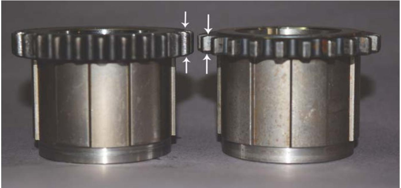
The new timing chain was narrowed down by about 0.100". You can see the difference in the gears.
