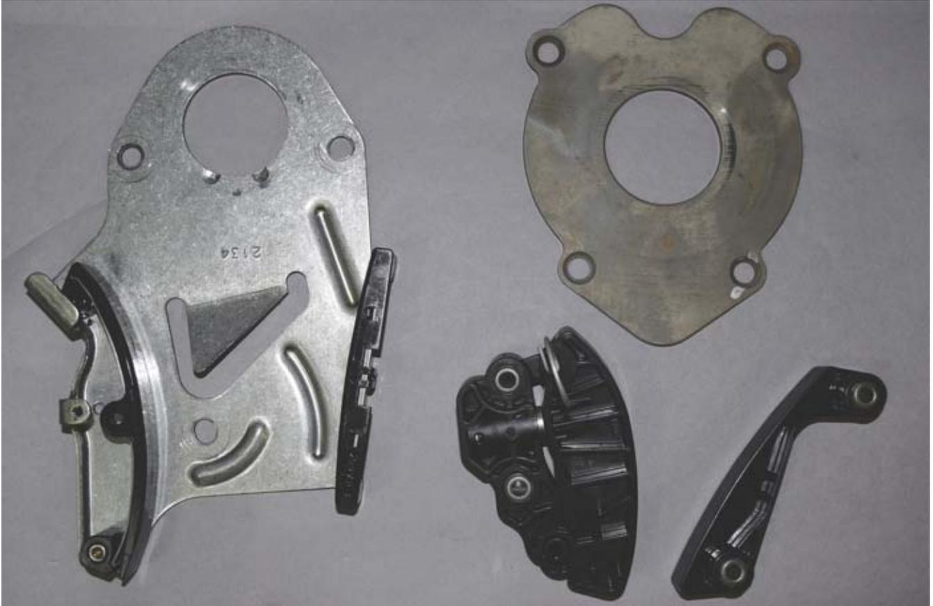
The original thrust plate that included the chain guide and tensioner was replaced by a separate thrust plate, a chain guide and a plastic tensioner with a spring-loaded piston.
