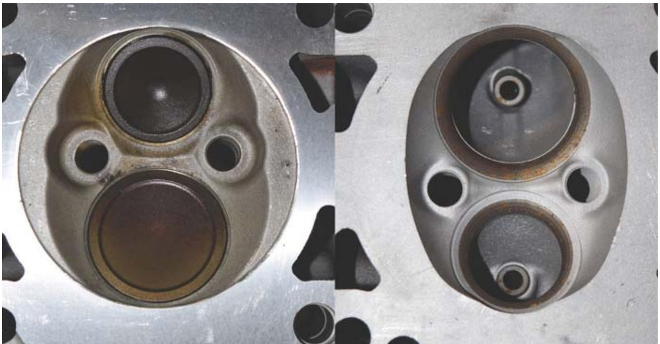
The new VVT heads (right) have 65cc oval chambers instead of the 85cc hemi chambers that were seen in the original Gen III heads.
