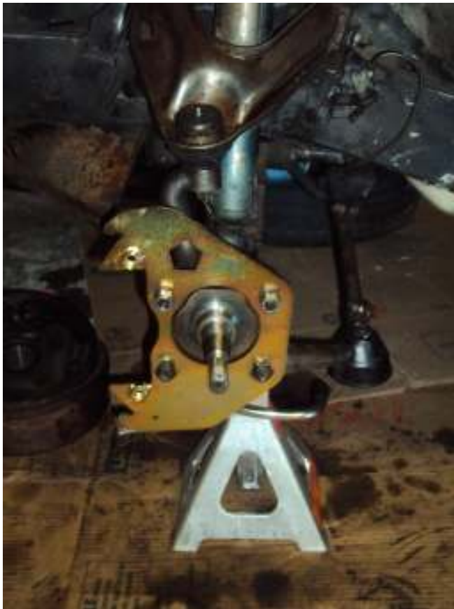
Scarebird adapter installed on driver's side.
