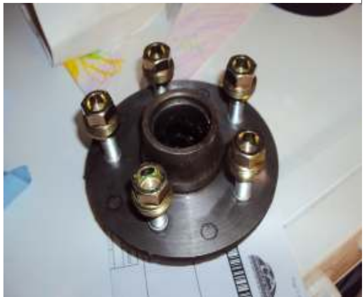
New studs installed in the hub. The machinist shaved a little off the surface of the hub for me to ensure a flusher fit with the rotor.
