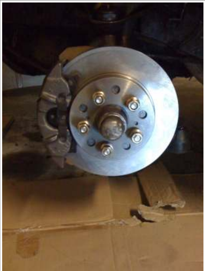
Caliper w/ pads installed and tested for proper fitting.
