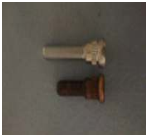
New Dorman stud on top, original on bottom
