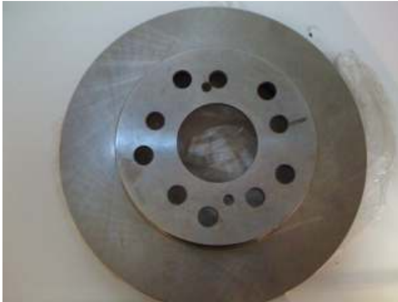
Hub re-drilled with the 5 x 4" bolt pattern
