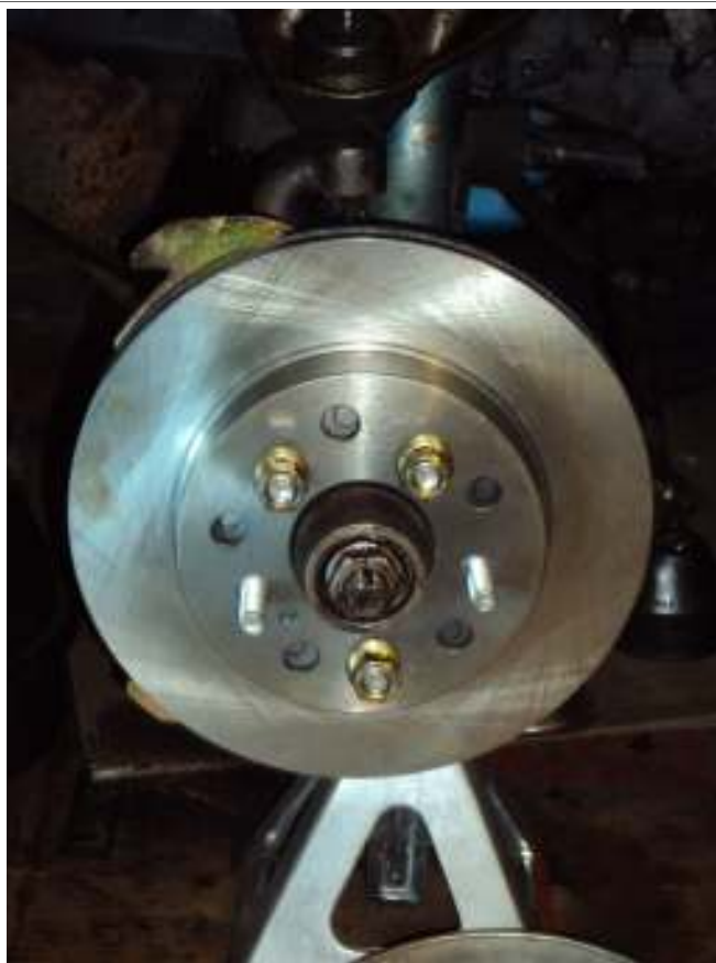
Rotor installed onto the hub and held in place with three lug nuts.
