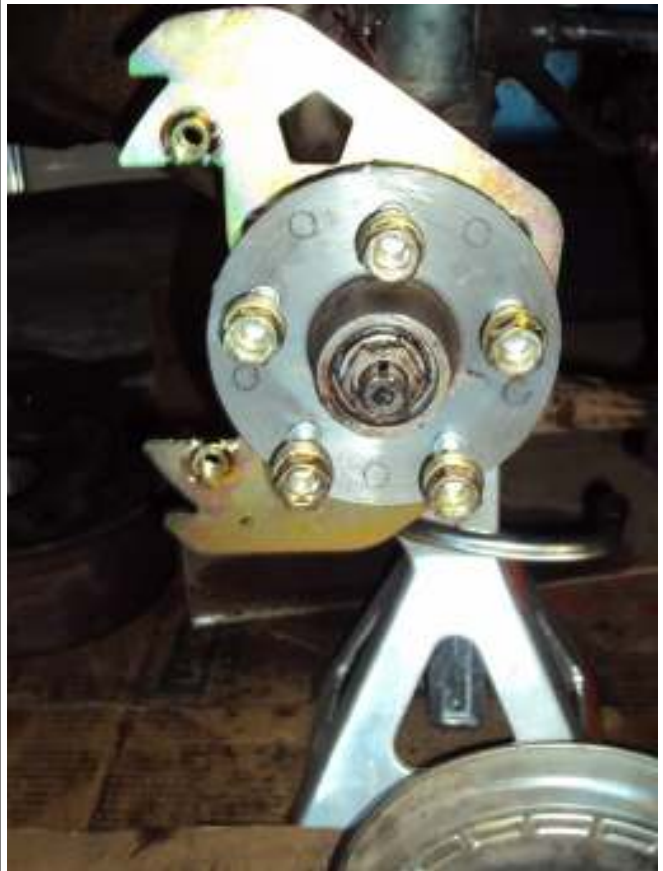
Rotor installed on spindle.
