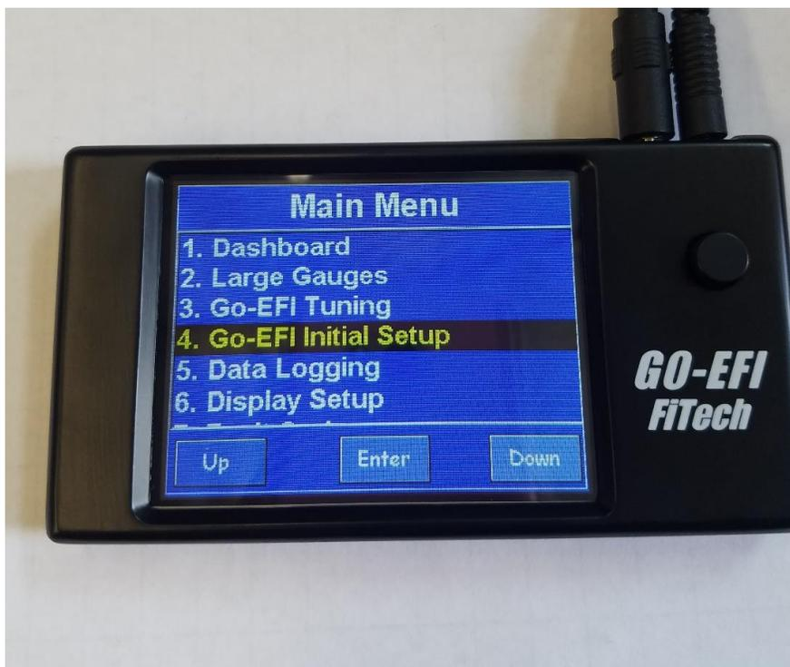
**Step 3:** go under option 1: engine setup. Then, scroll down to option 6 (pump PWM/FCC) and select edit, press clear (CLR) and enter a new value. The lower the number the slower the pump will run. **If you have a Fuel Command Center the best value to set this feature to is 40.** Press ok, then in the fuel pump control menu press the center of the control stick to send the change to ECU.
