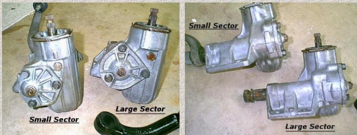
Notice the various differences between the two castings. Most notable is the cover plate, which makes it possible to tell the difference by just glancing under the hood in the junkyard.
