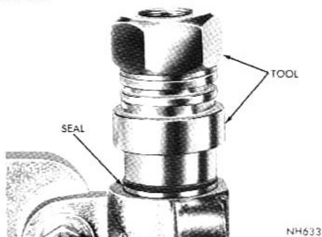
Fig. 6—Installing Cross Shaft Inner Oil Seal
