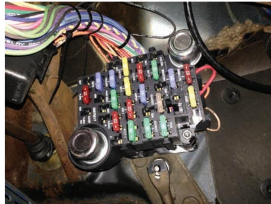
Fuse Block mounted under Dash in 1974 Duster
