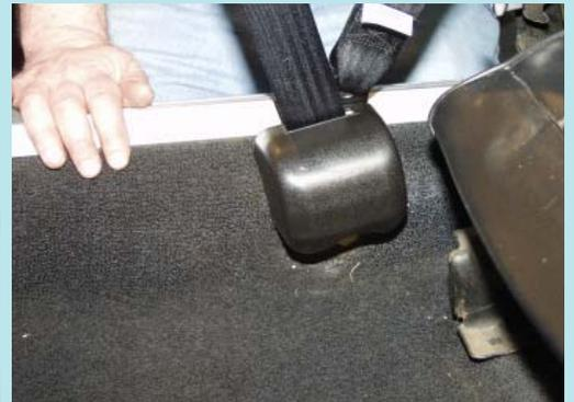
The shoulder anchor gets mounted behind and angled forward of the retractor. On the E-Body pulling and smoothing the carpet will get you a professional looking install.
