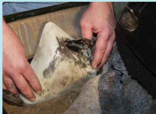
On the E, you need to remove the trim bezel and lift the carpet exposing the retractor cover.
