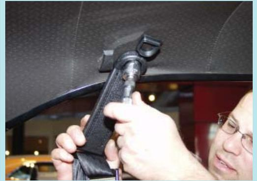
Install the shoulder mount of the three point harness and securely tighten.
