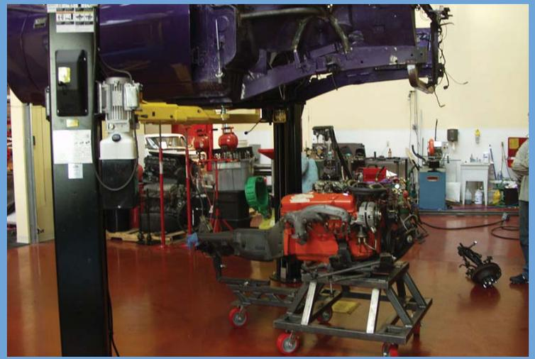
We next need to remove the drivetrain and front suspension. After removing the brakes, shocks, control arms and spindles, we position our engine cradle in place. The engine cradle supports the engine, mounted on its K-member and the transmission so they can be removed as a complete assembly. Once in position, we lift the car body away from the drivetrain. The new setup will be installed in the same way, just like at the factory.
