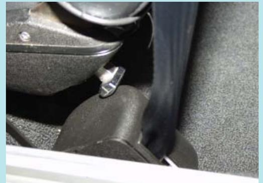
A-Body seat knob needed to be removed to push the seat all the way back.
