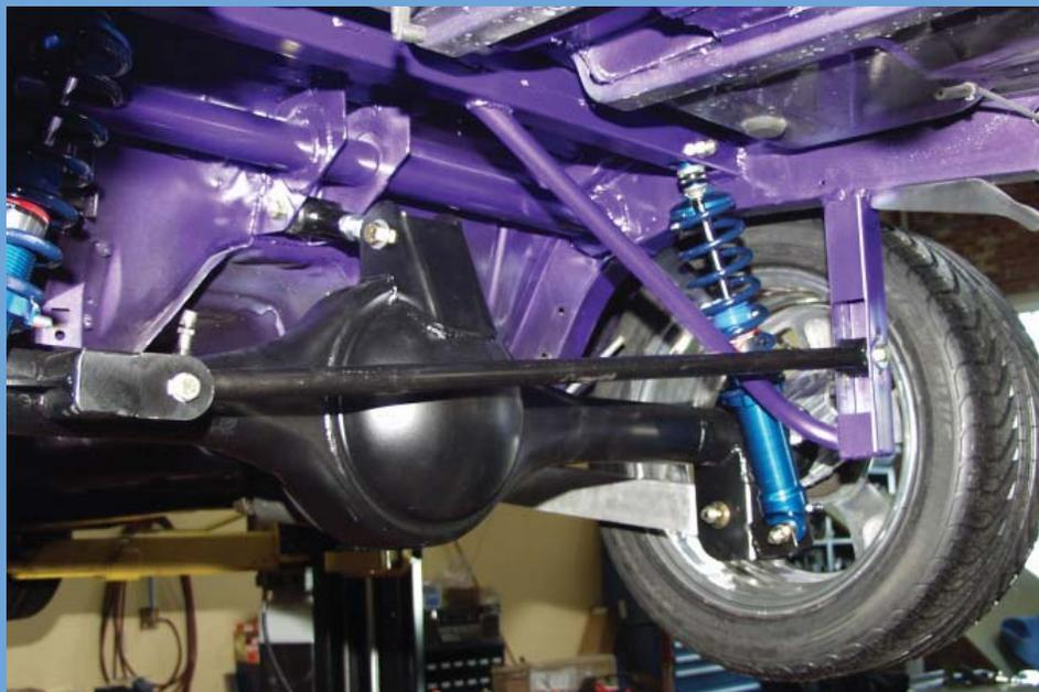
Here are some pictures of the rear suspension fully installed. Panhard bar frame mount is supported by a J-Bar brace tied to the upper coilover mount. The upper coilover mount has a filler plate in its center that ties the mount to the structure of the car at its center.
