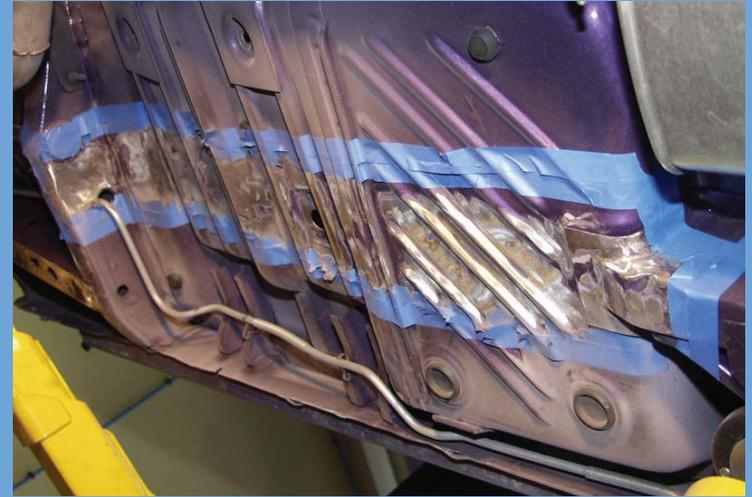
We start the installation of our Laser Cut Subframe Connectors. As you can see in the first picture these will tie the car together from the rear frame rails to the transmission/T-Bar cross member. After we test fit them, the floor pan is masked and paint sanded off in preparation for welding. The picture on the right shows what these look like after the floor pan has been re-painted.
