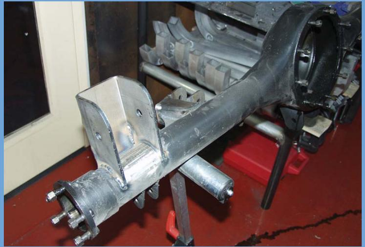
The fuel tank, rear axle, leaf springs and shackles are all removed. The factory stamped steel upper shock mount will also be removed as it is not strong enough for coilover shocks. The car's rear axle housing is disassembled and welded in place are the trailing arm mounts, panhard bar mount, third link mount, lower coilover mounts and rear sway bar mounts.
