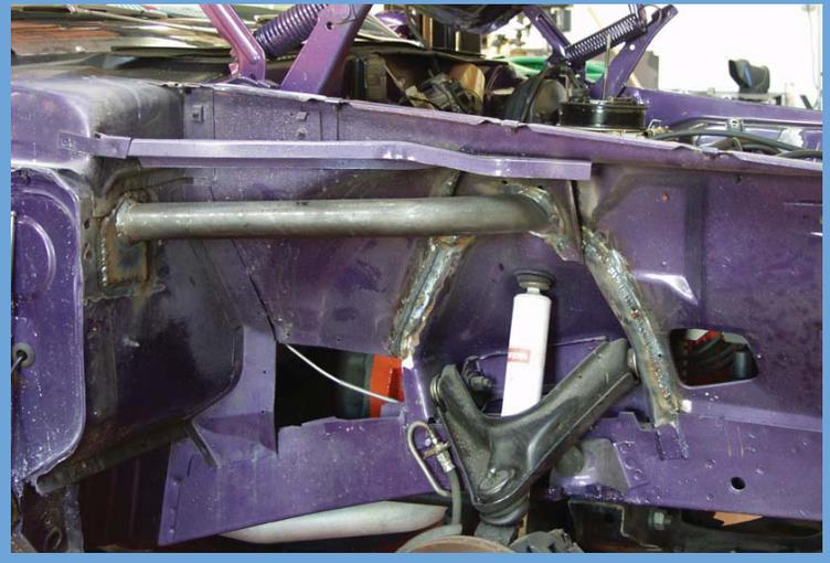
We begin installing Inner Fender Braces which tie the car together from the shock tower to the firewall. There are laser cut gussets that reinforce the factory support brackets that the tube is welded to above the shock tower (pic on left has it installed and on right not yet installed). Also note that we seam weld the perimeter of the factory shock tower as this is only spot welded from the factory. Also note the light-weight stamped factory support above our piece.
