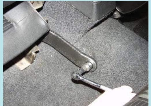
Install the short end of the new three point belt that has the push button release and tighten securely. For the E-Body with a console, install it parallel to the console and then rotate it up.
