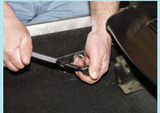
Start removing the outer belt down by the door. For an E-Body Start with the sill plate.
