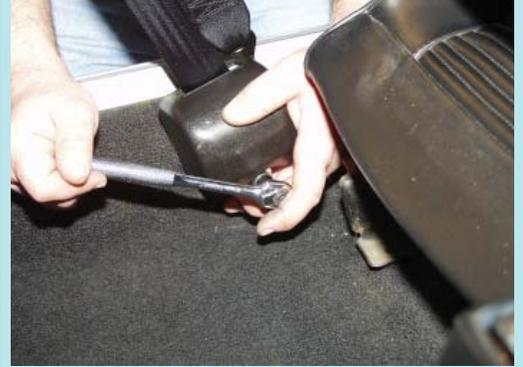
Install the new retractor and shoulder anchor in place. The anchor gets mounted behind and angled forward of the retractor.
