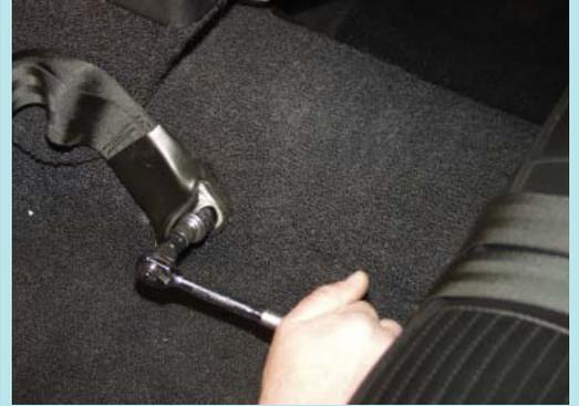
First slide the front seats all the way forward. Remove the factory inner belt from its mount on the transmission tunnel.
