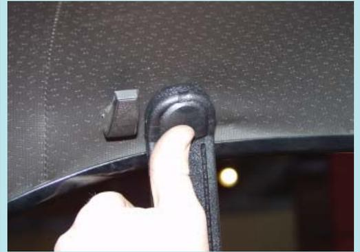
Press the trim cap in place to cover the bolt.
