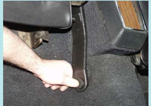
Finish the inner portion of the belt by pressing in place the bolt trim cover.
