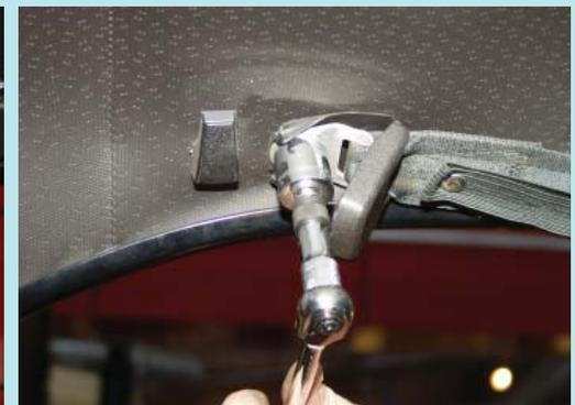
Next, remove the factory shoulder restraint by prying open the trim cover and then removing the bolt.
