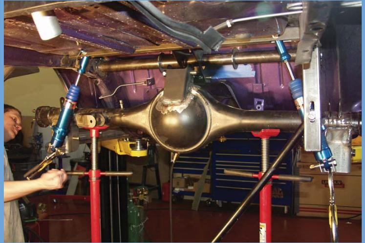
After carefully measuring, the new upper coilover mount is the first piece to be tacked in place. All measurements are checked and positioned and tacked in place. This includes the panhard bar frame mount, third link chassis mount and rear anti-roll bar axle tube.
