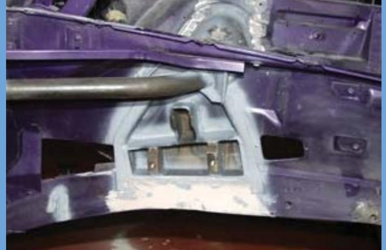
This car is getting the XV Level II Suspension System installed front and rear. Starting at the front, we need to install the Upper Control Arm and Upper Shock Mount Assembly, which comes as a welded assembly in the kit as shown on the left. The assembly fits directly into the shock tower and is then welded in place to the shock tower and frame rail.
